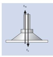
The theoretical value in N at a vacuum of -0.6 bar (at sea level). Depending on the operating conditions, this value may have to be reduced in order to take the necessary safety factor, the losses due to friction or a lower vacuum value (due, for example, to a porous workpiece).
