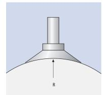
This specifies the minimum radius at which the workpiece can be gripped securely by the suction pad.
