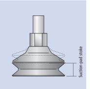
This is the lifting effect which occurs during evacuation of the suction pad.
